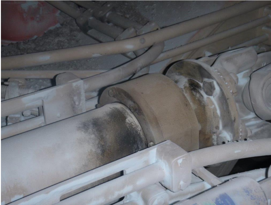
Figure 3 Heat damage to an underground haul truck
