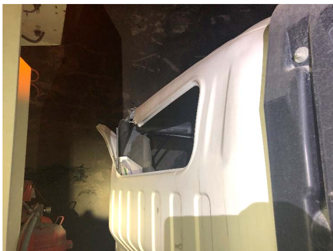
Figure 6 and 7 (left) Post-incident simulation of the drill steel entering the truck cabin from the Jumbo. (right) Damage to the back of the cabin body above the passenger seat caused by the drill steel entering the cabin (IncNot 0034365)
