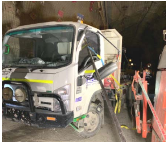
Figure 6 and 7 (left) Post-incident simulation of the drill steel entering the truck cabin from the Jumbo. (right) Damage to the back of the cabin body above the passenger seat caused by the drill steel entering the cabin (IncNot 0034365)
