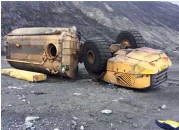
Figure 1: The water truck that rolled over.
