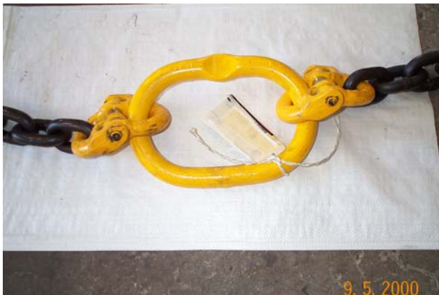
Photo 1: Acceptable assembly using chain connectors.
