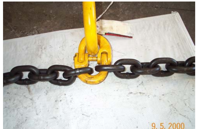
Photo 2: Avoid this chain connector assembly arrangement, because the connector is not designed for side loading.
