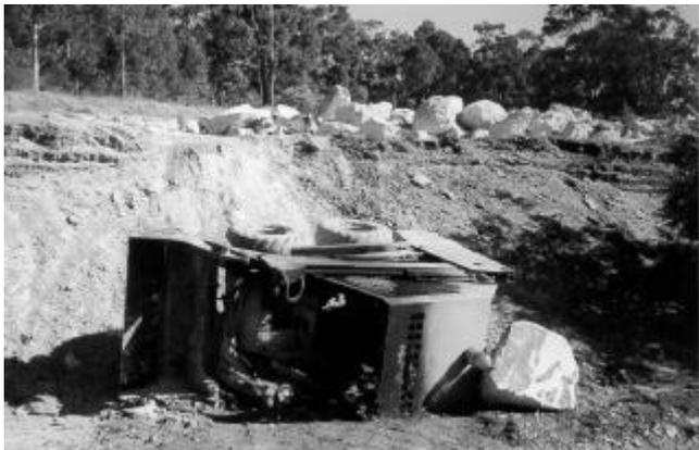
The photo shows the Bobcat lying on its side at the bottom of the slope. The large stone next to it may have rolled down the slope and contributed to the accident.
