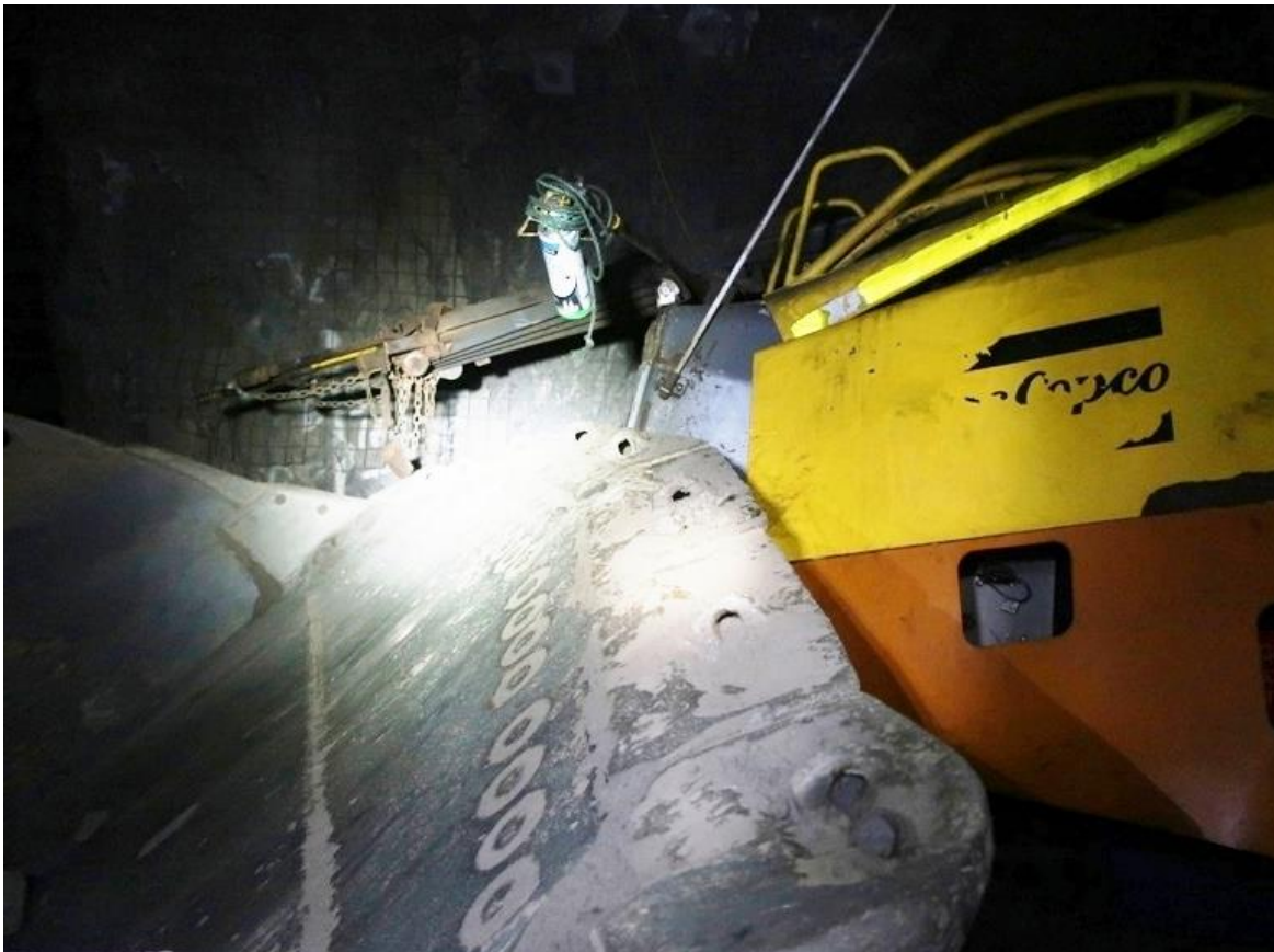
Figure 2. Impact point of the loader and jumbo
