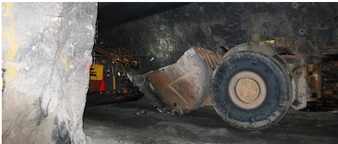
Figure 3. Access drive and impact point of the loader and jumbo
