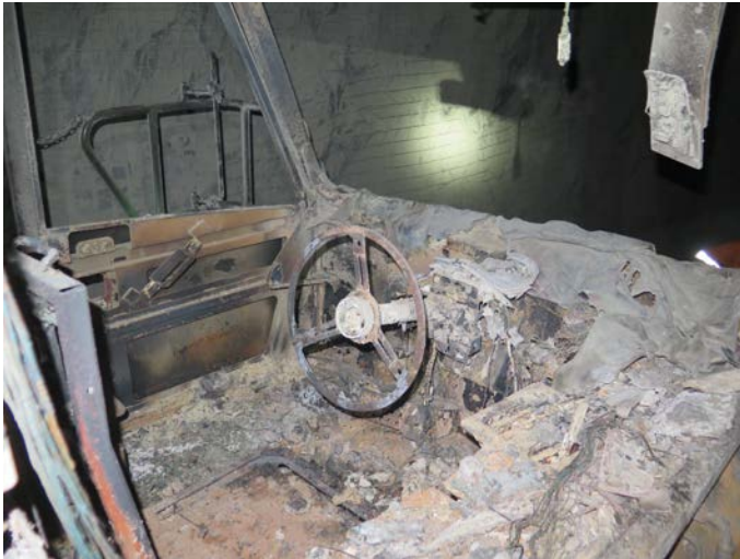
Figure 4: Non-metallic materials in cabin affected by fire
