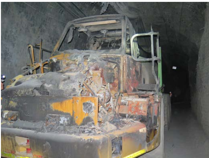
Figure 3: Damage to the burnt guards and bonnet
