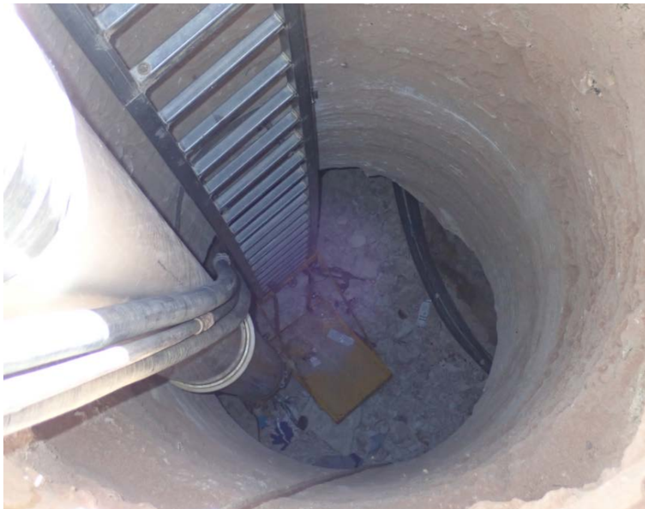
Photograph 3: View of the base of the shaft showing the access ladder and where the opal miner fell. (Photograph by Resources Regulator)
