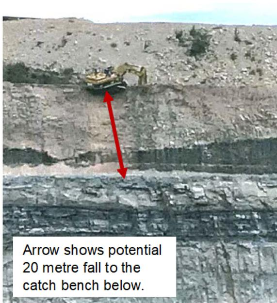
**Photograph 2: View from the bench of the excavator rotated over the edge of the highwall. (Photograph by Resources Regulator)**
