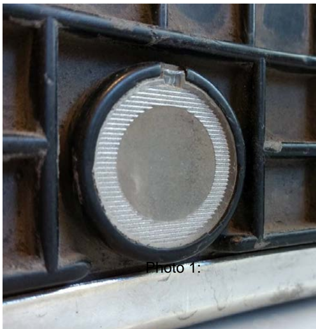
Photo 1: Dirt obscuring the moisture indicator.
