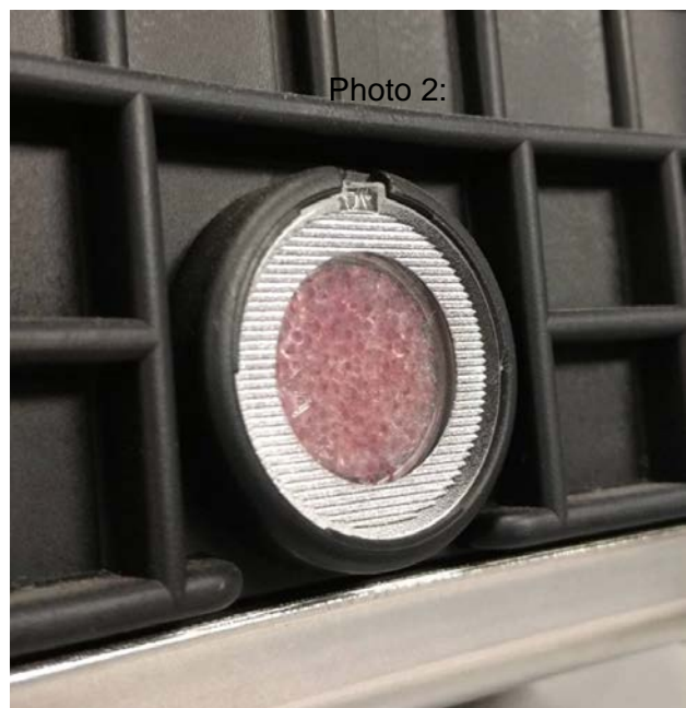
Photo 2: Clean window with moisture indicator visible.
