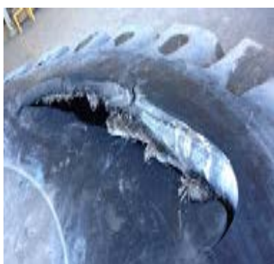
Photo 2: Sidewall slit in the tyre
