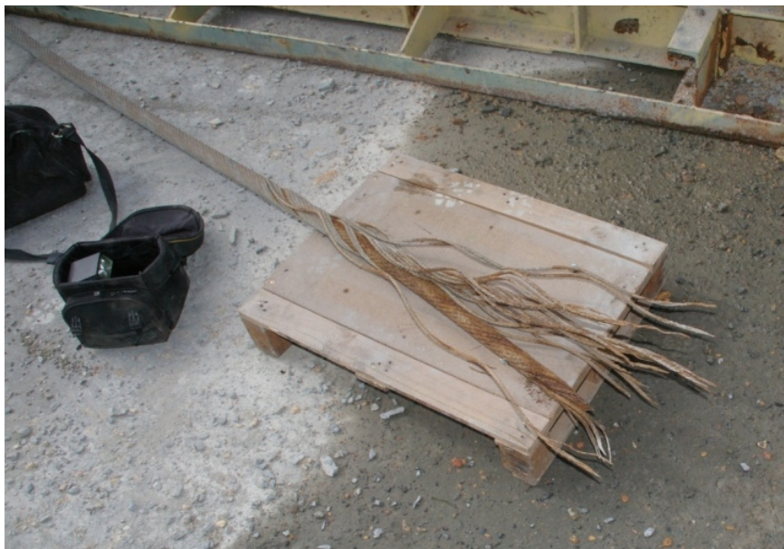
Photo 1 - Broken end of balance rope.
