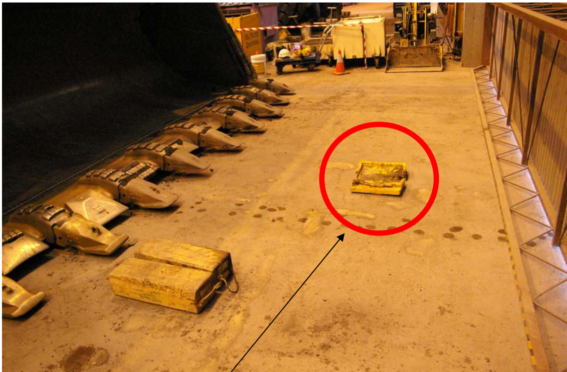
The polyurethane workshop floor pad (circled) that was ejected from beneath the front end loader bucket.
