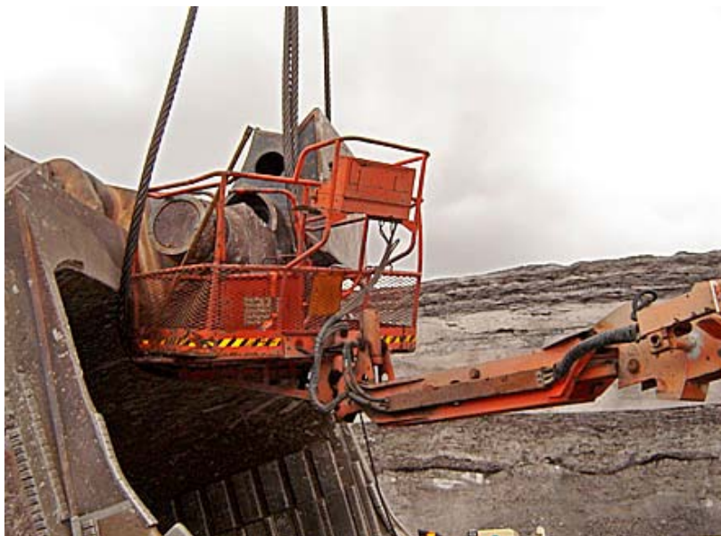
The elevating work platform after being propelled into the bucket of the P&H 4100
