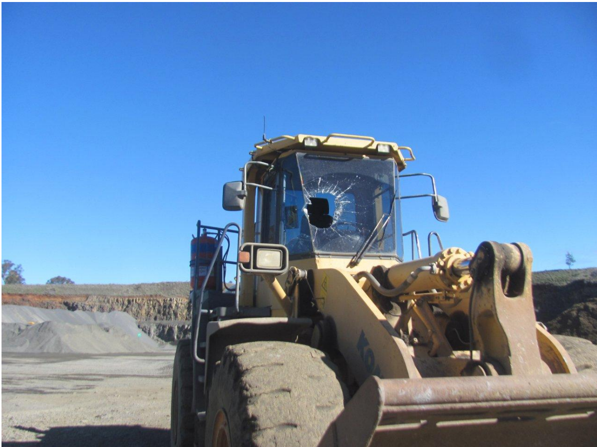
Figure 1: Damage to the loader windscreen. Photo by Mine Safety
