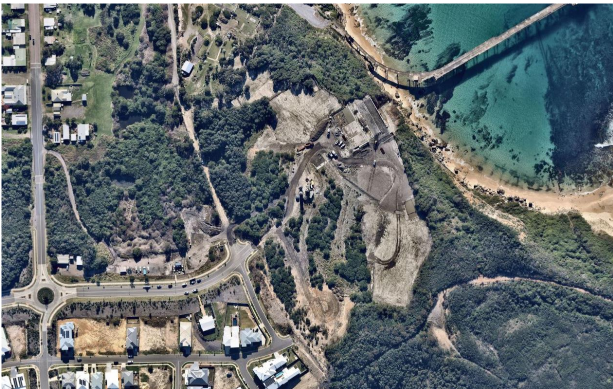
Figure 7: Domains 1A, 2A and 4A in June 2020 showing installation of fill material within the coal bin site. Fill material included crushed concrete (generated on site), flyash, cement, grout and excess material generated from bioremediation works
