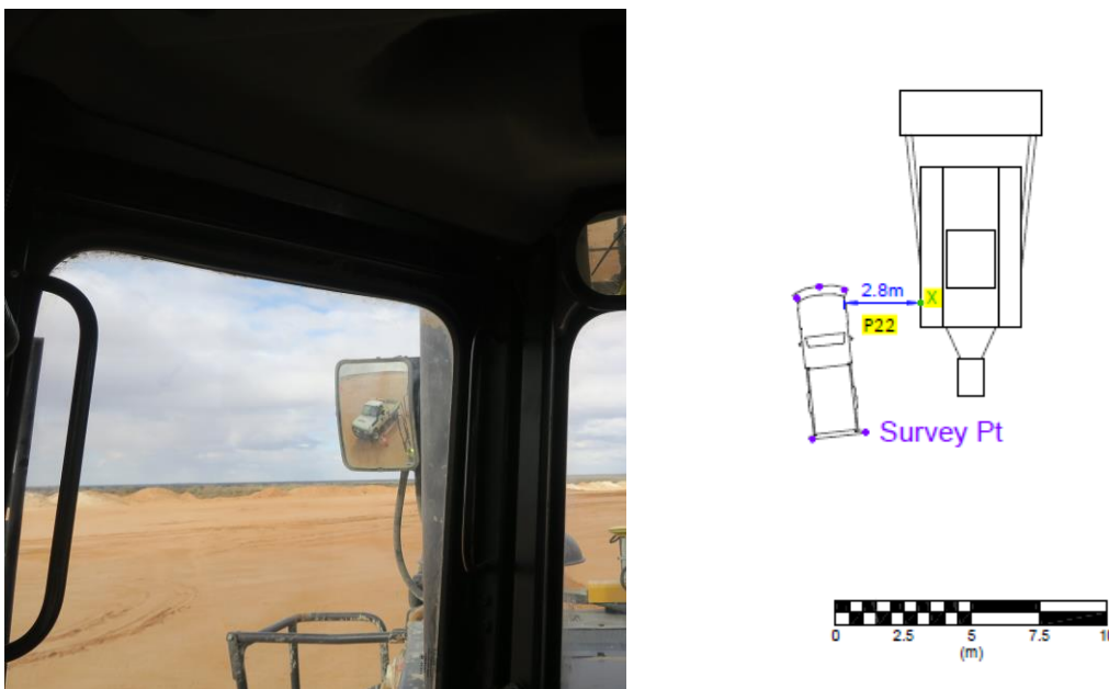
Figure 13: BSL Caterpillar D10T dozer 902 side mirror view of light vehicle
