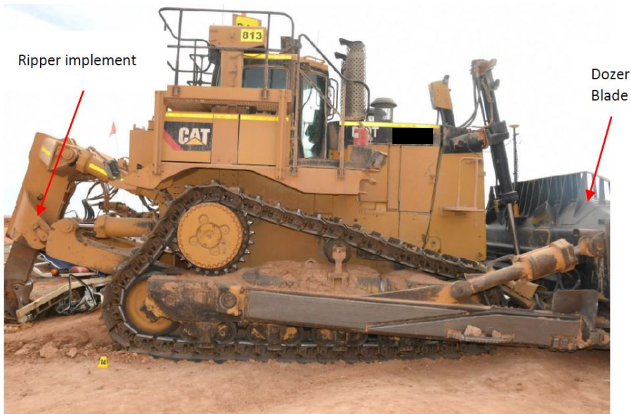
Figure 1: Caterpillar D10T dozer DZ 813
