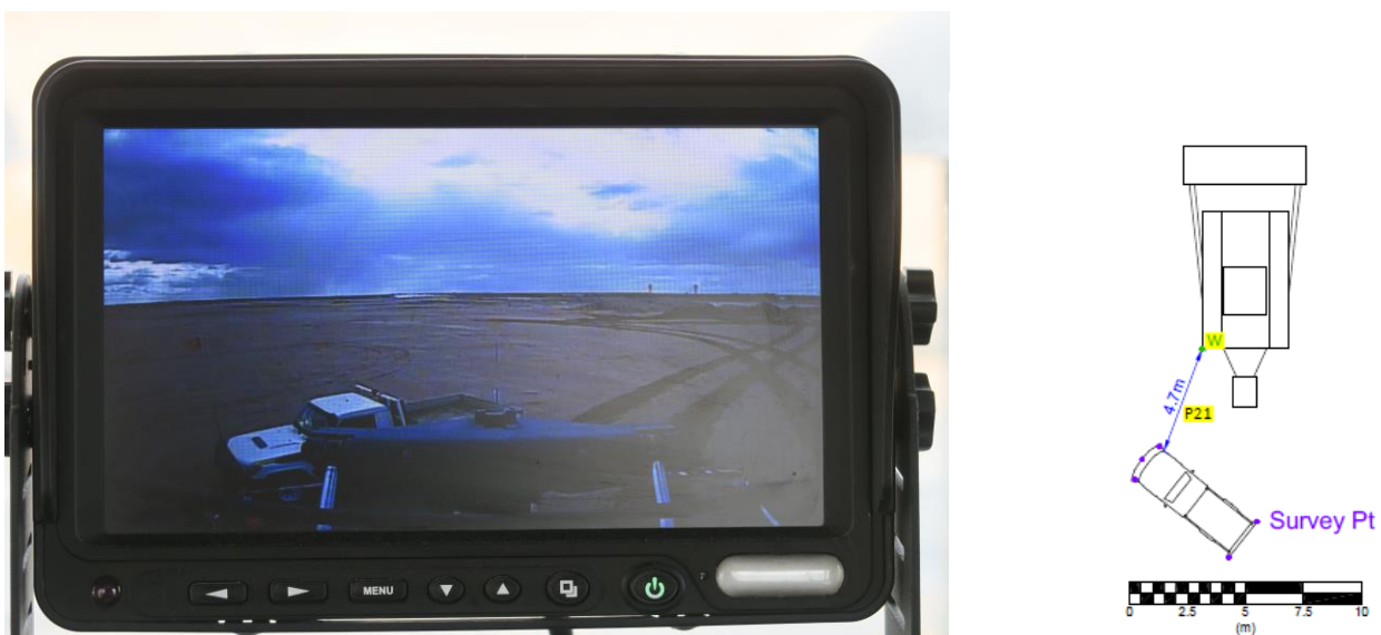
Figure 12: BSL Caterpillar D10T dozer 902 reversing camera view of light vehicle
