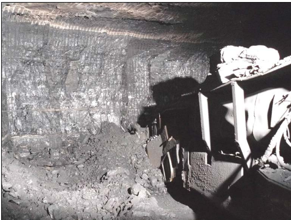
Photograph 19 Looking into the first right hand rib pocket showing the extent of over width extracted against the continuous miner.
