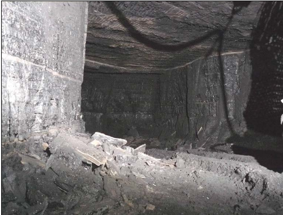
Photograph 13 Looking into the left hand rib pocket that had been extracted by Mr Jones before extracting the right hand pocket. First left hand pocket in B Heading between 5 and 6 cut-through.
