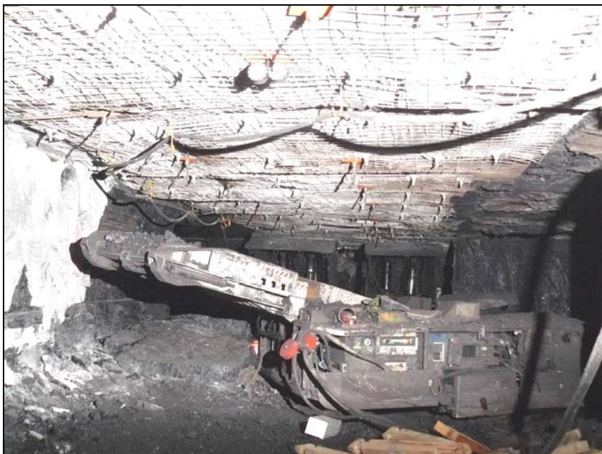
Photograph 4 Looking inbye of the continuous miner in the right hand side pocket and the fallen rib coal inbye of the continuous miner boom.
