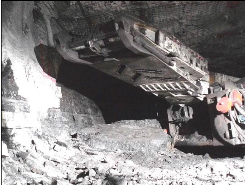
Photograph 5 Looking inbye of the fallen slab inbye of the continuous miner boom.
