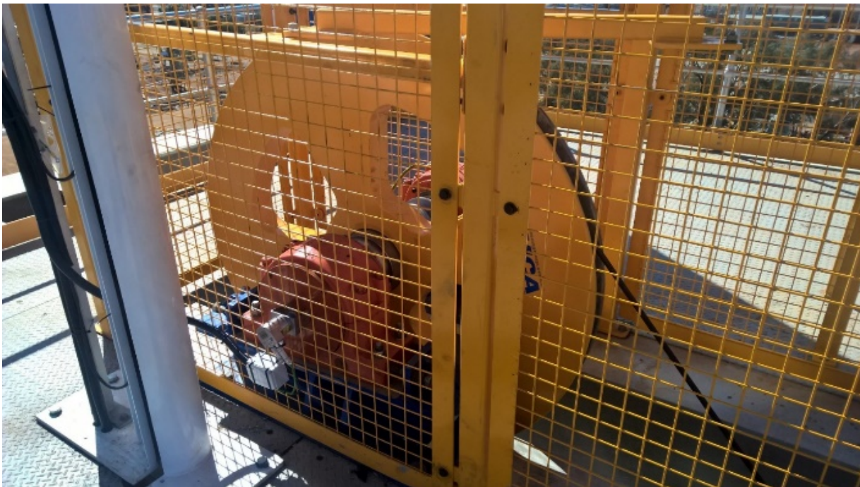
Figure 14 Typical headsheave on a shaft sinking winder
