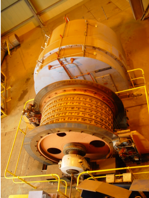
Figure 9 Friction winder drive arrangement
