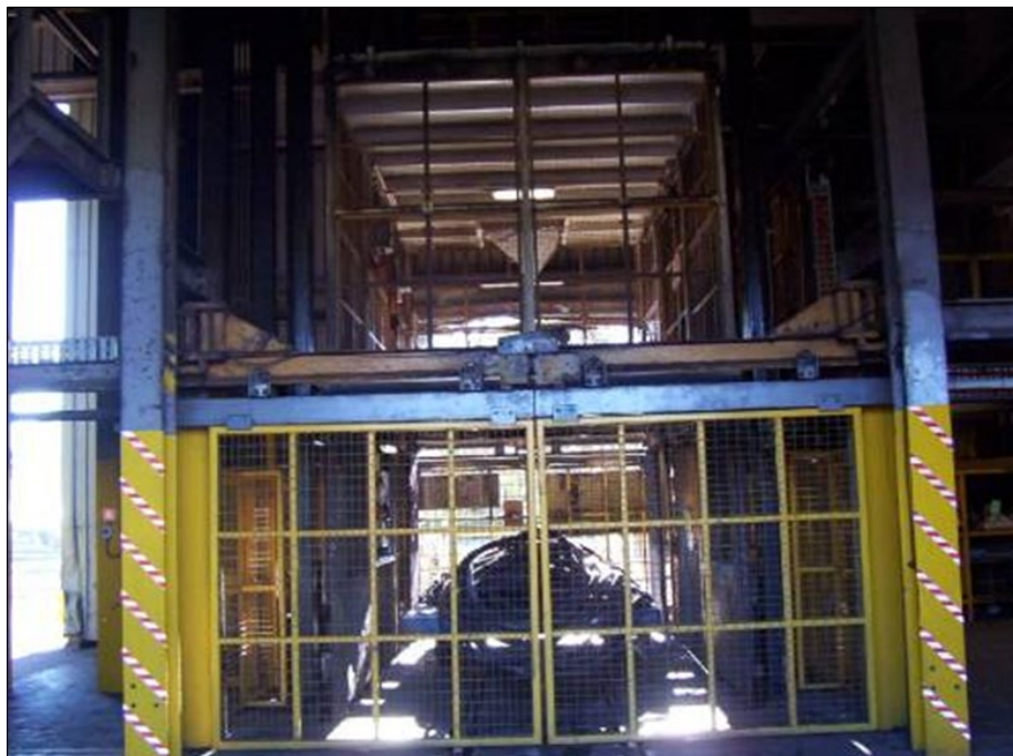
Figure 7 Tower-mounted friction winder house
