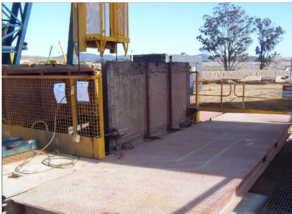
Figure 19 Shaft top doors in open position
