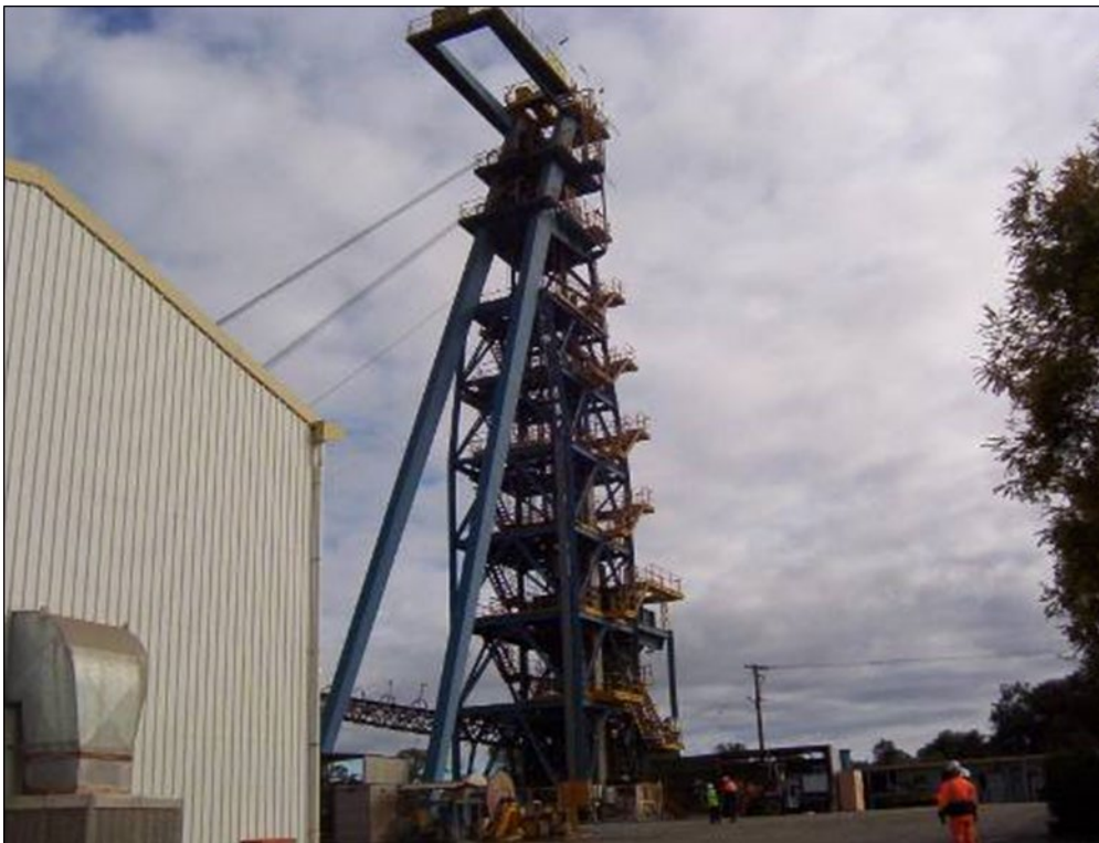
Figure 29 Ground-mounted friction winder house, ropes and headframe
