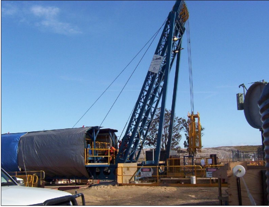
Figure 12 Headframe for a typical stage winder
