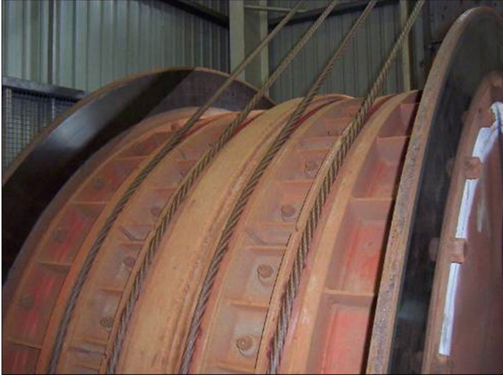
Figure 29 Ground-mounted friction winder house, ropes and headframe
