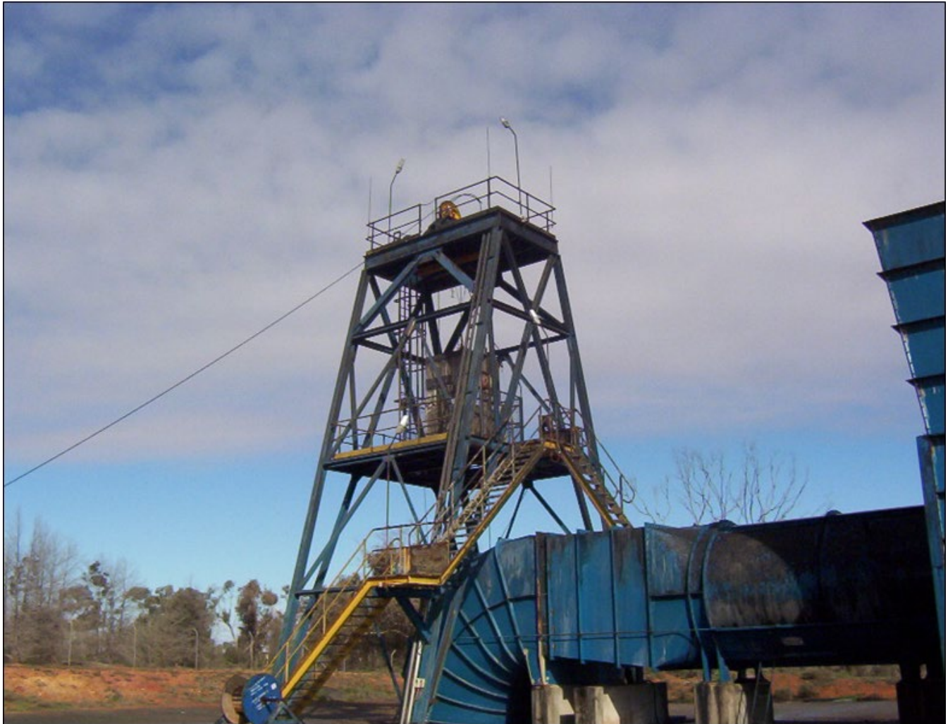
Figure 3 Single drum personnel winder - Shaft top installation
