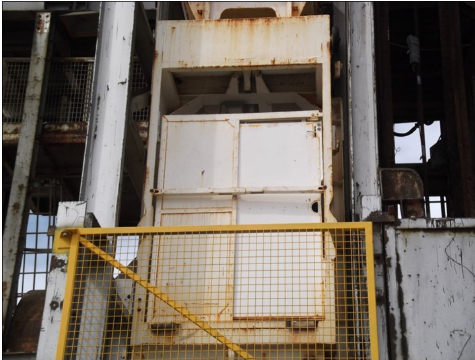
Figure 26 Vertical shaft personnel riding conveyance
