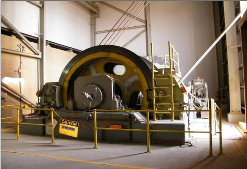
Figure 24 Tower mounted friction winder showing two brake paths
