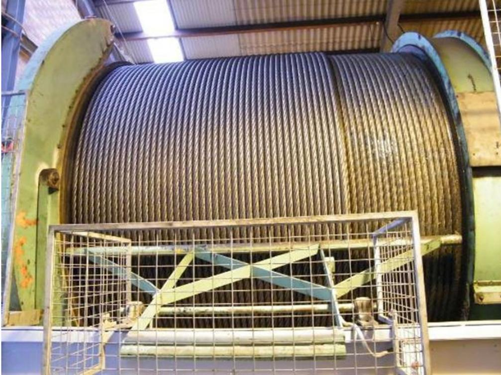
Figure 2 Older spoked, stiff winder drum design
