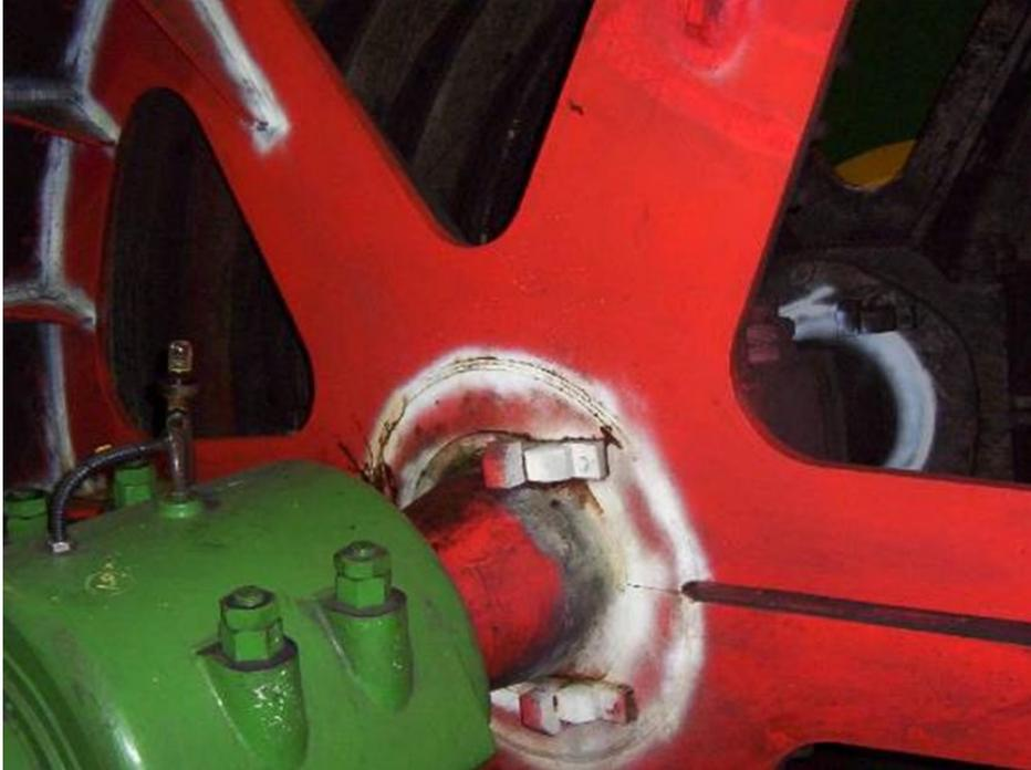
Figure 6 Drum shaft attachment - Bolted arrangement
