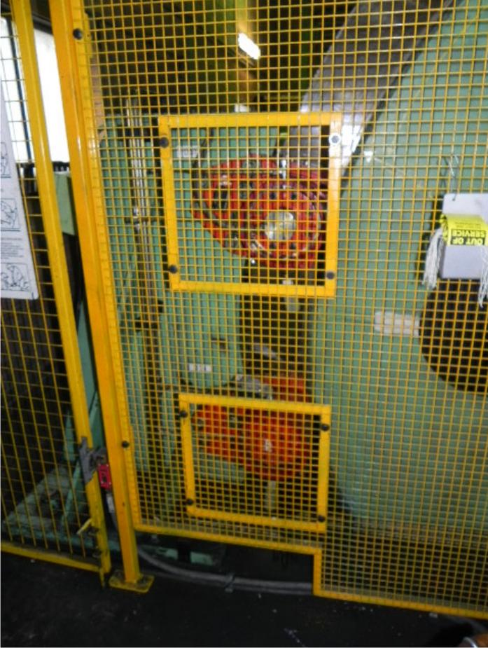
Figure 22 Drift haulage winder low speed brake, disc and caliper arrangement
