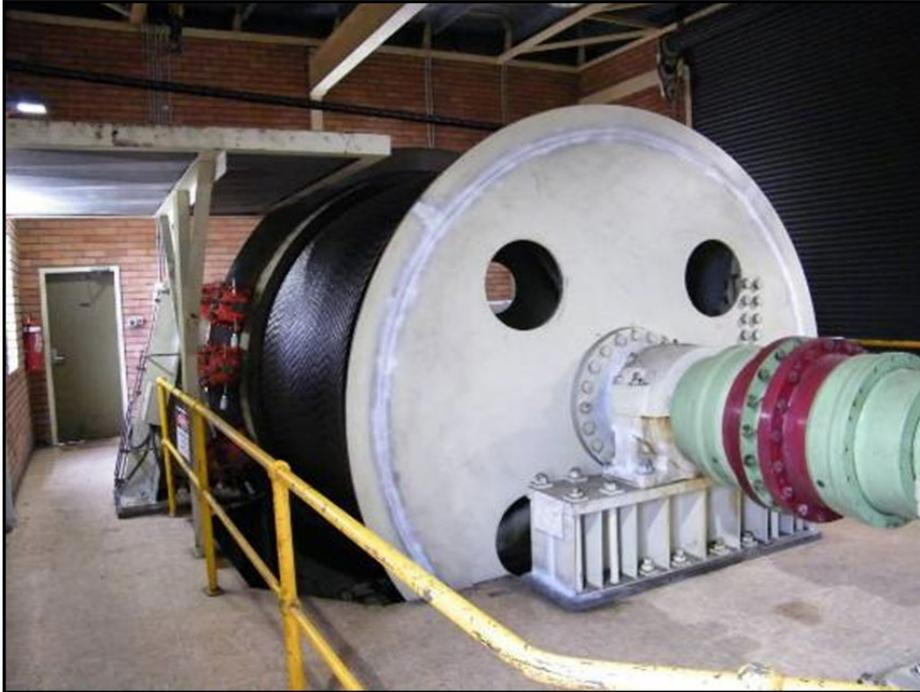
Figure 8 Non-coupling end of drum shaft for 80 tonne drift haulage
