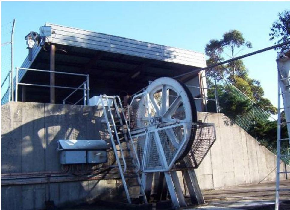
Figure 15 Headsheave installation - ground mounted friction winder
