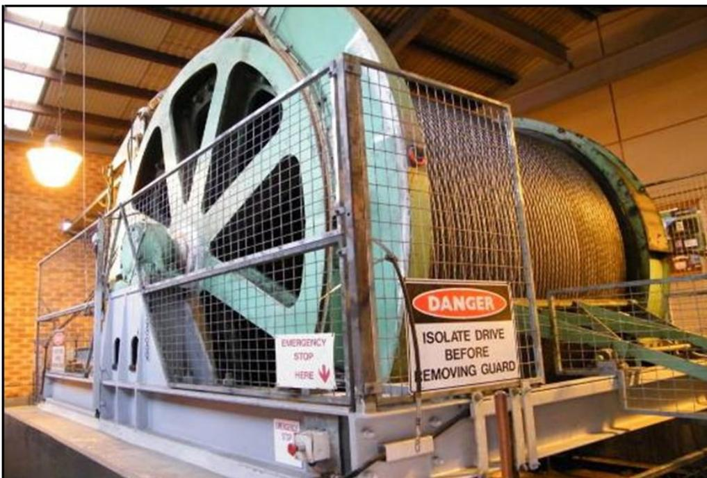
Figure 3 Flexible fabricated drum design
