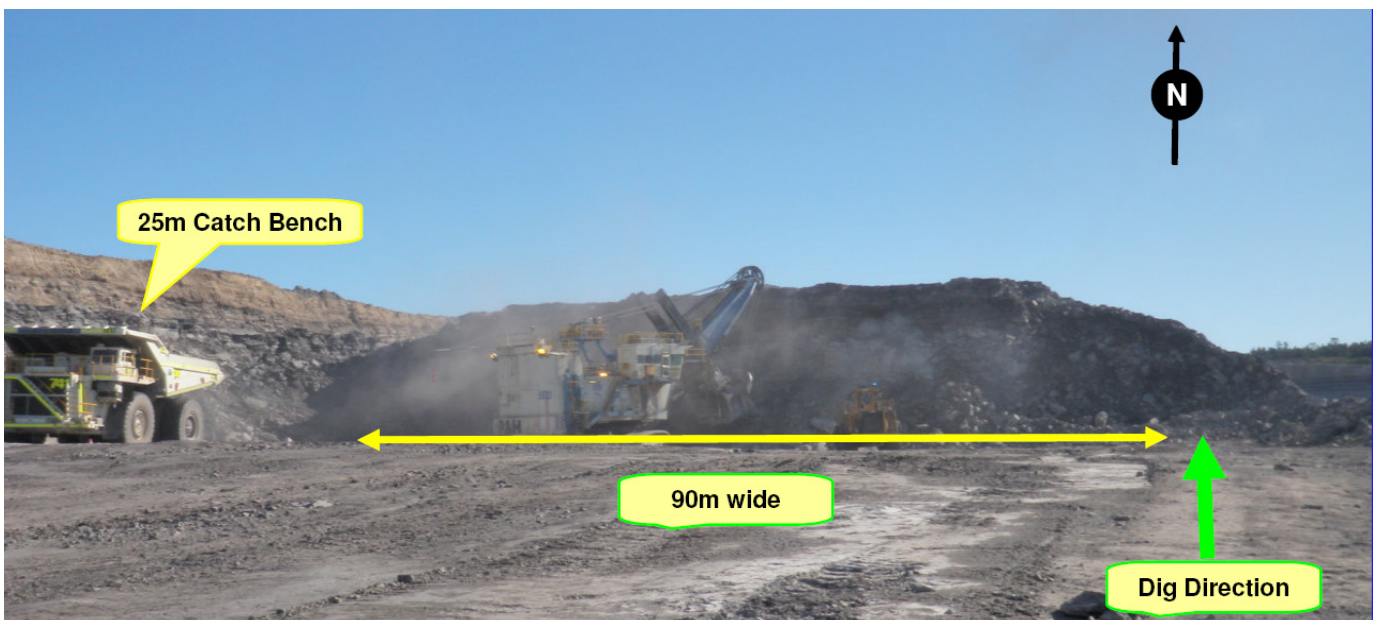
Photograph 1: Overburden being removed by shovel and trucks 2 .
