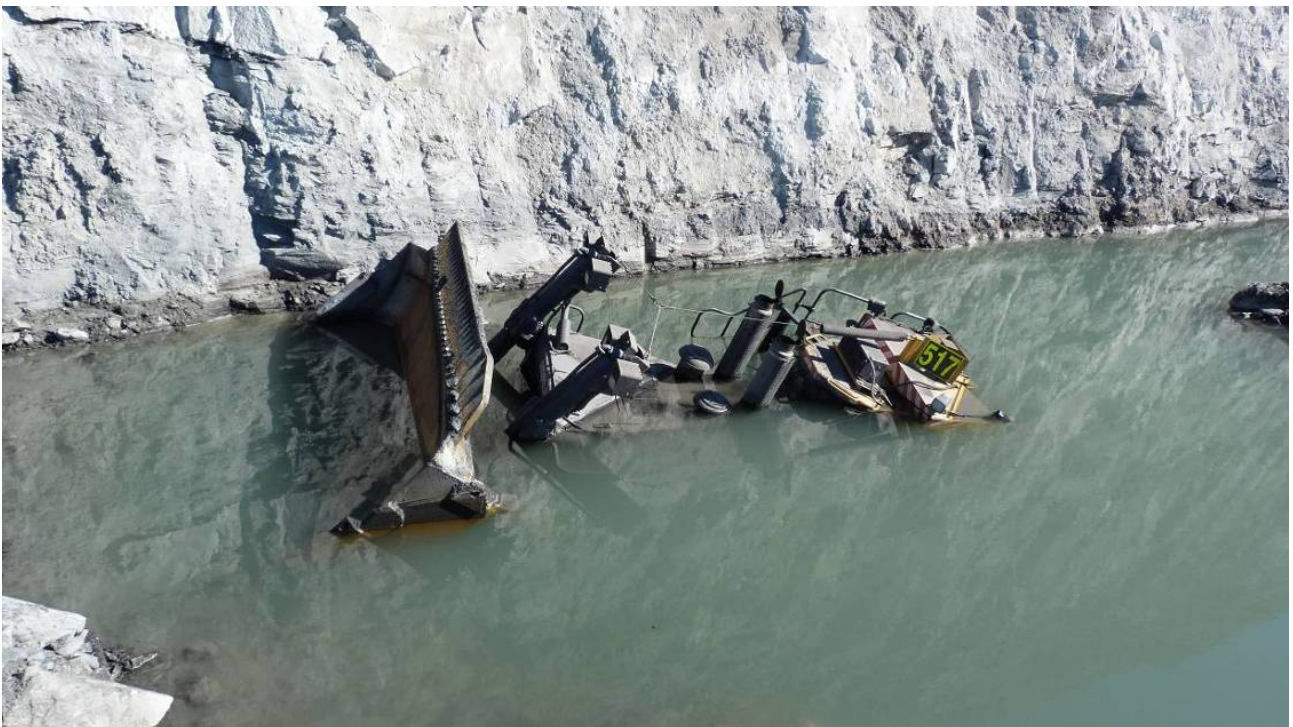
Photograph 6: CAT D11T dozer submerged in the sump.
