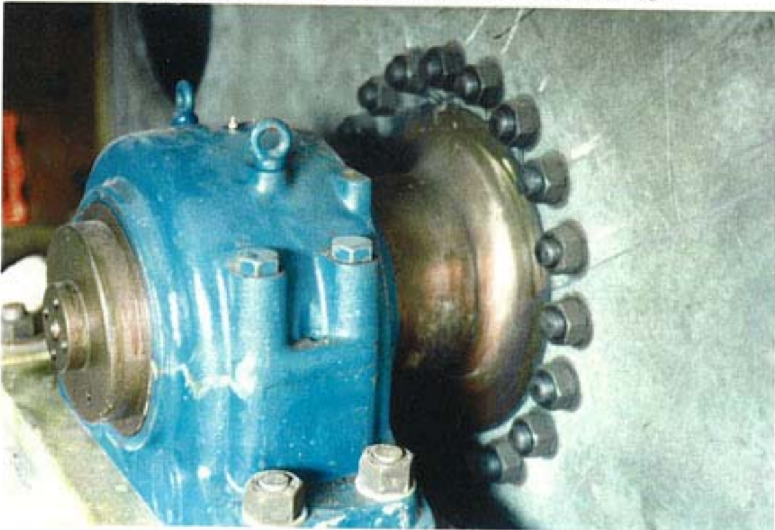
Non-Coupling end of drum shaft for 80 Tonne drift haulage
