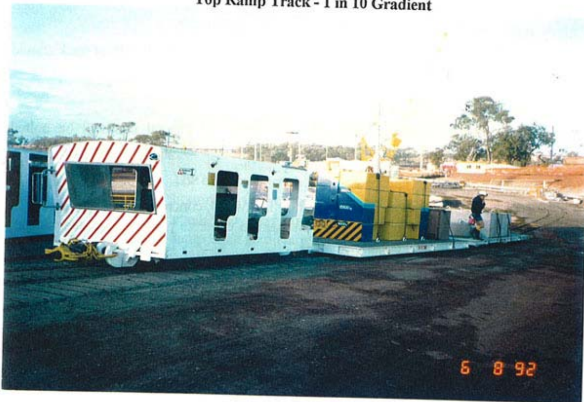
Control car with loaded flat-tops - Maximum end of rope load 108 Tonnes
