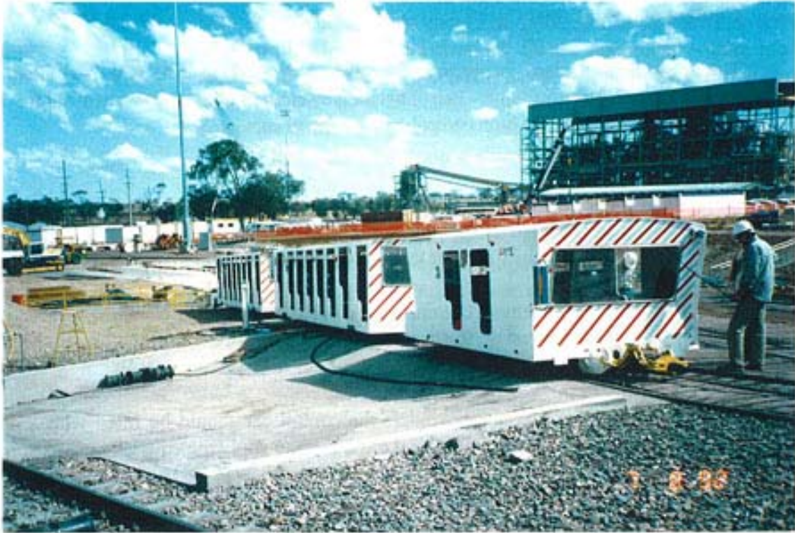
Drift haulage control and personnel cars (Man Transport System)
