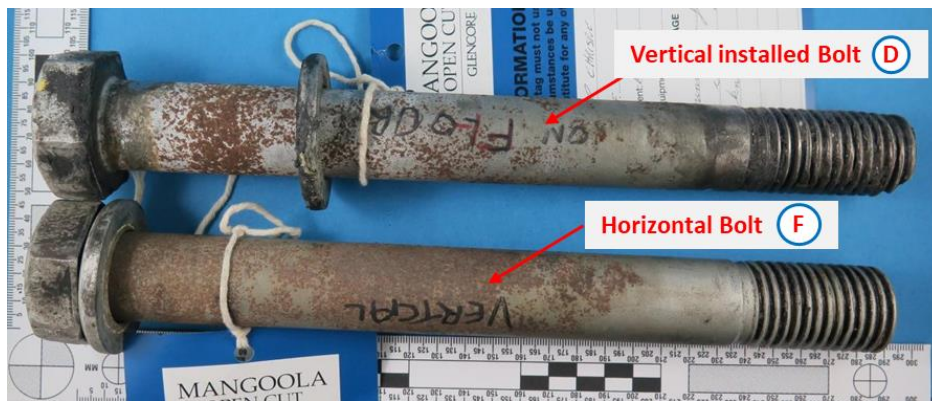
Figure 4-1: Two Bolts Examined by BV
