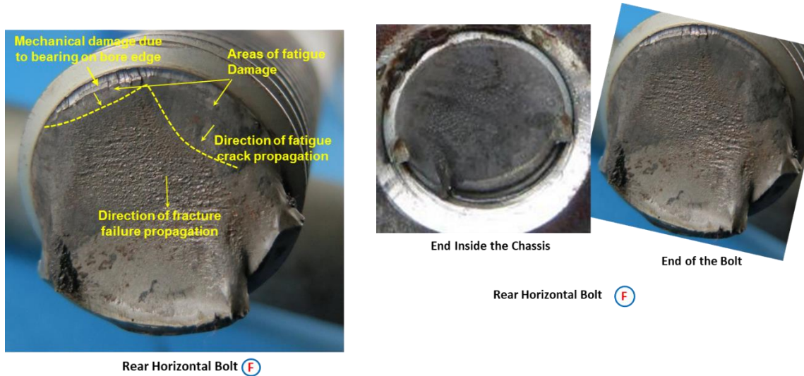
Figure 4-7: Fracture Surface of Rear Horizontal Bolt F
