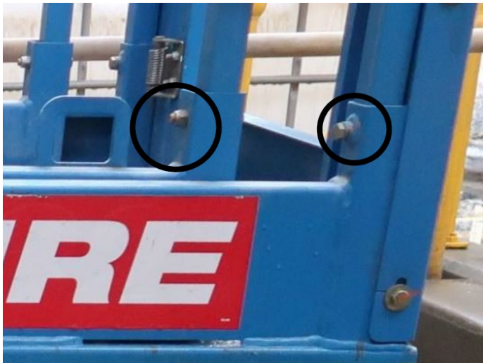
Figure 4 Bolting system used to fix guardrail panels
