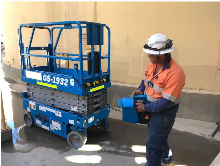
Figure 8 Operator 'walking' a GS1932 scissor lift using wired controller
