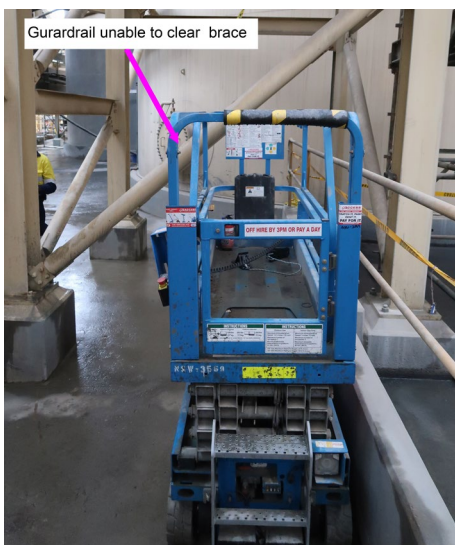
Figure 12 Approximate location of scissor lift when the worker attempted to move it under the brace
