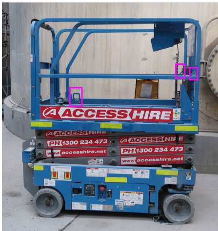
Figure 5 Personal fall protection anchor points on scissor lift
