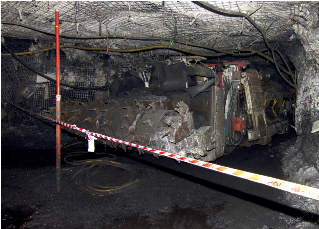
Figure 29 CM 35 after being moved from the incident; note rib guard is bent into the machine, the inflection measuring 110 mm. 82
