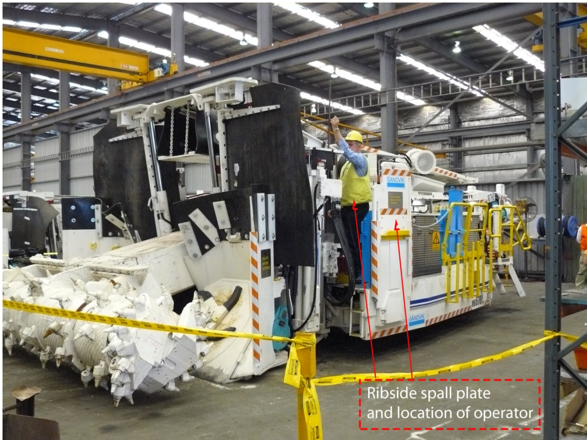
Figure 3 ABM 25 cutting drum and left-hand side of bolter miner. Picture by Investigation Unit (April 2008).
