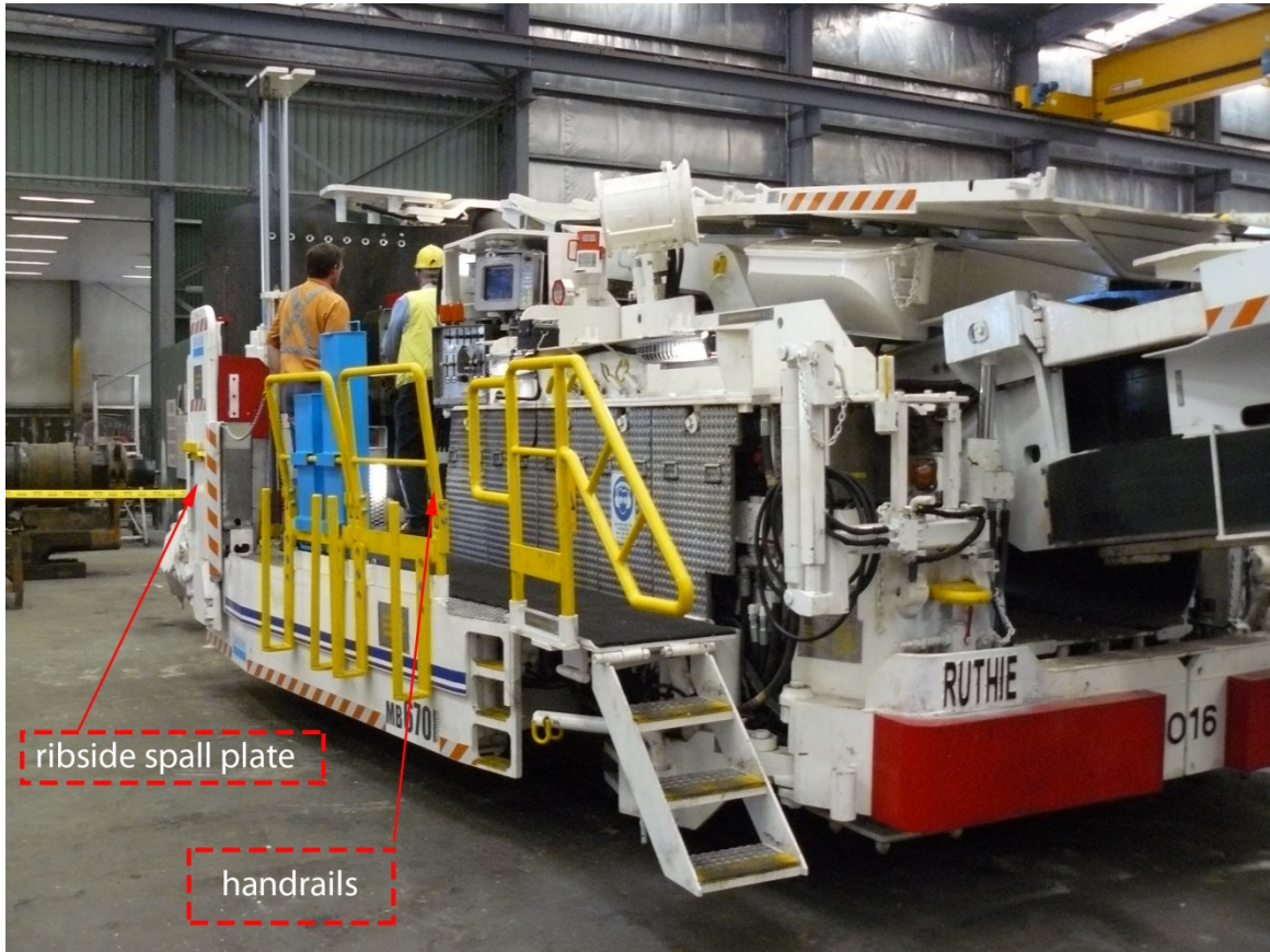
Figure 4 Left-hand side of ABM 25 bolter miner from rear of miner. Picture by Investigation Unit (April 2008).
