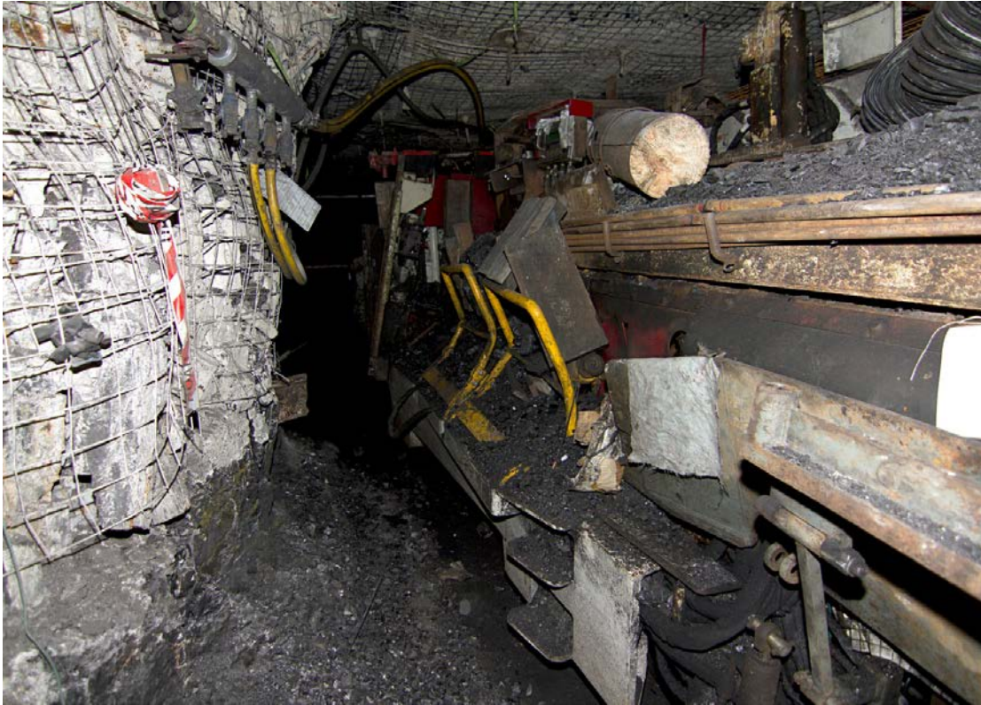
Figure 29 CM 35 after being moved from the incident; note rib guard is bent into the machine, the inflection measuring 110 mm. 82
