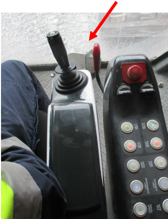
Figure 5: Hydraulic isolation - pilot control shut-off lever located beside the excavator operator's seat
