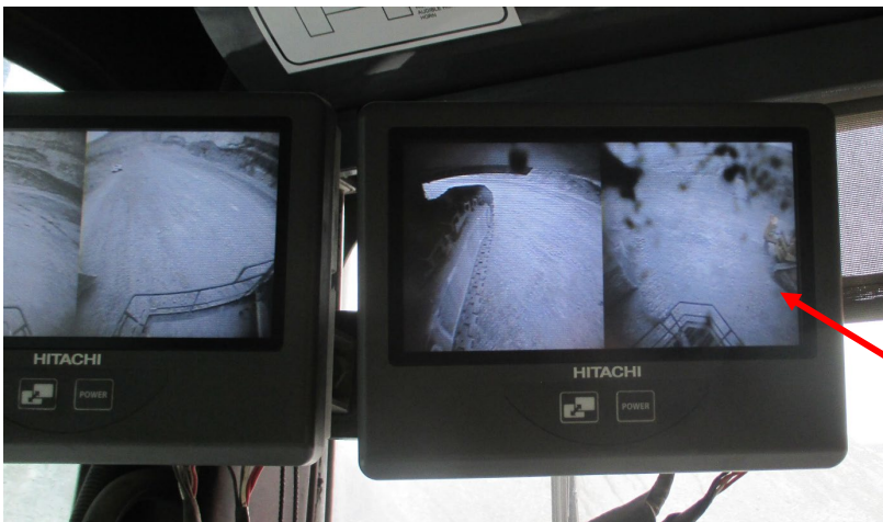
Figure 4: Two display screens in the excavator cabin depicting camera views of what could have been displayed at the time of the incident.
