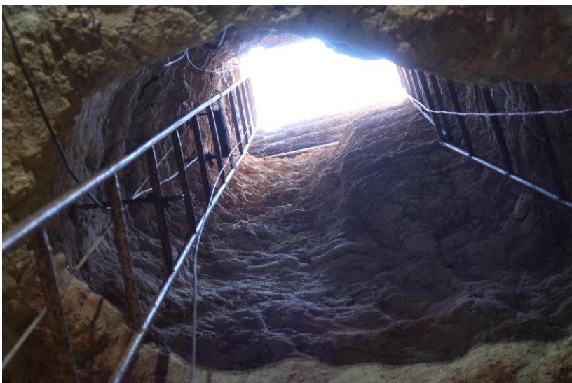
Figure 2 Material hoist shaft at the opal mine
