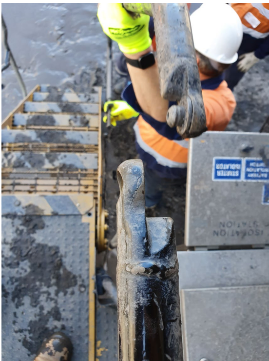
Figure 2 Failed handrail from initial incident
