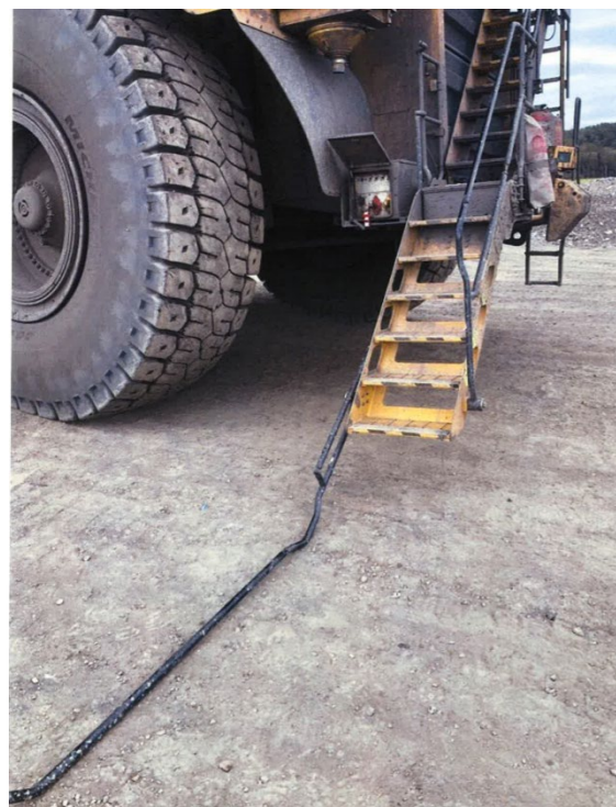
Figure 3 Failed handrail from second incident
