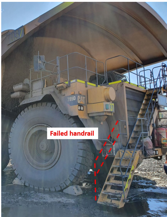
Figure 1 Failed handrail on haul truck
