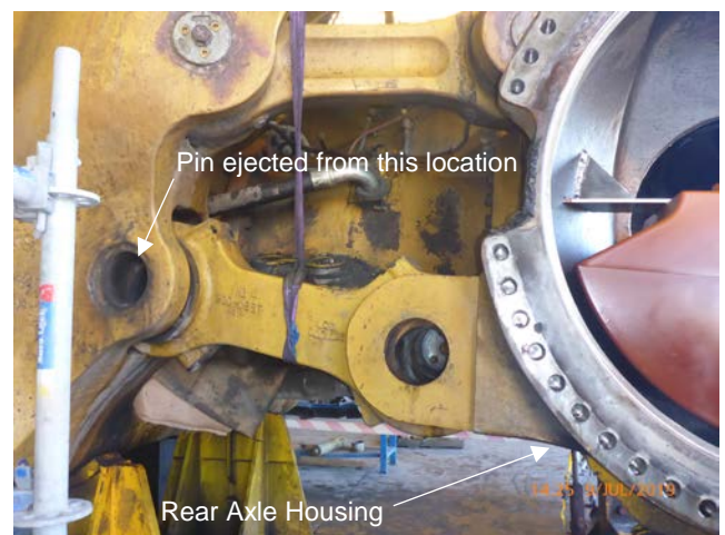
Figure 2 Lower Suspension Link (Dogbone) supported by crane as preserved following the incident
