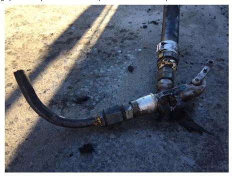
Photograph 2: Fuel splash filler nozzle adaptor attached to Banlaw quick connect fuel nozzle.
