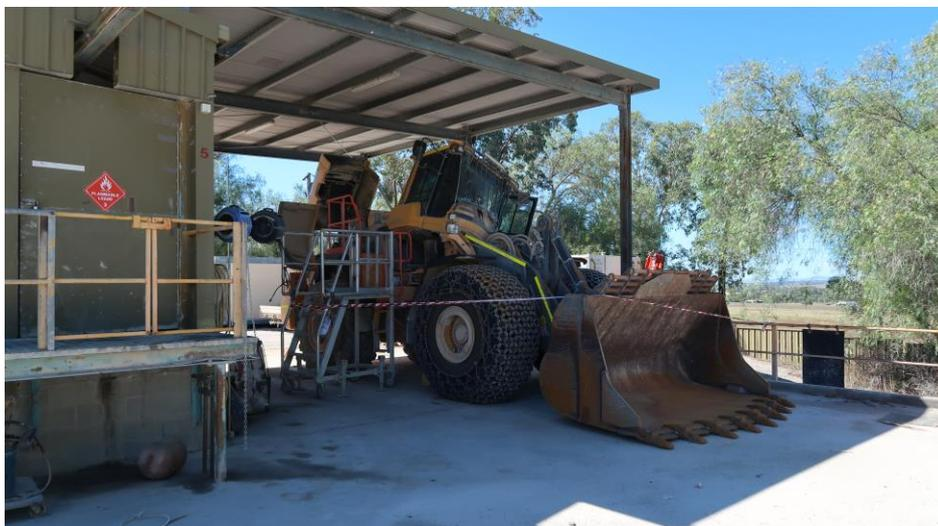
*Figure 2 Position of the worker after the cabin was raised and a wooden chock provided by mine workers during the release of the worker*
