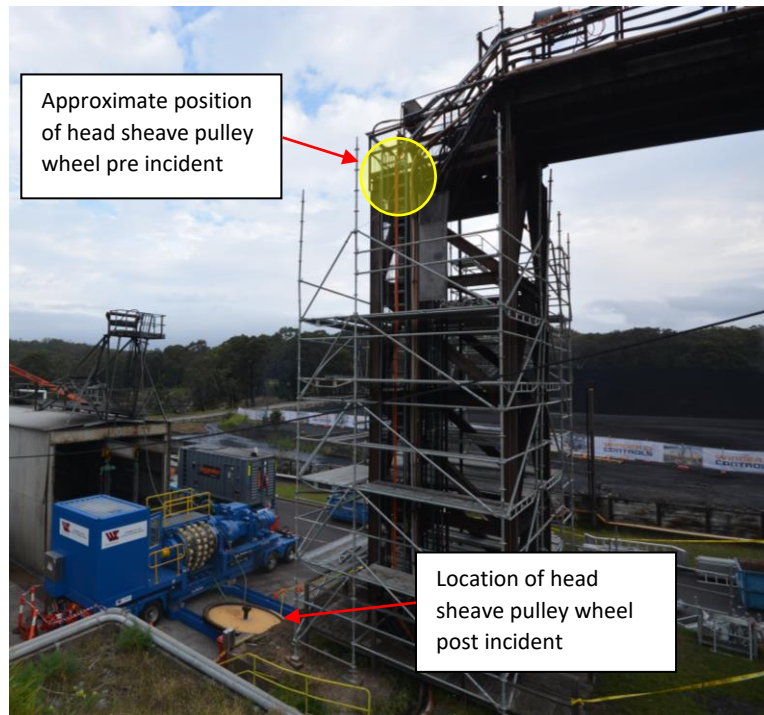
Figure 3 Damaged head sheave pulley wheel assembly components
