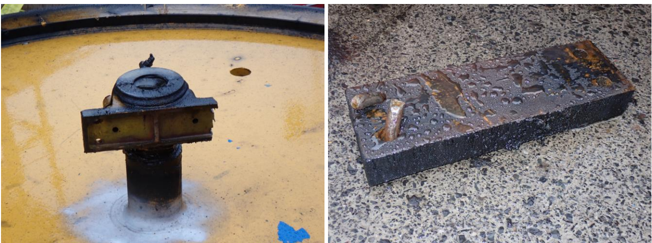
Figure 3 Damaged head sheave pulley wheel assembly components
