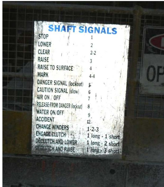
The shaft signalling system did not encompass a specific signal identifying when people were riding in the kibble in accordance with recommended industry practice. Accordingly there was no way for the winder driver to know that Mr Junk was in the kibble when the incident occurred.
