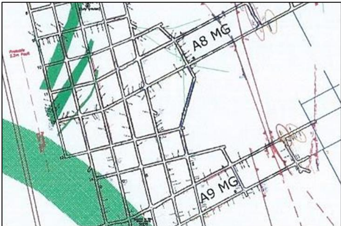
Figure 5: Plan view showing continuous miner position relative to face and burst location.
