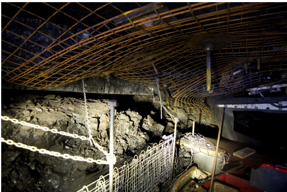
Figure 8: Close-up of burst coal pile adjacent to the continuous miner.
