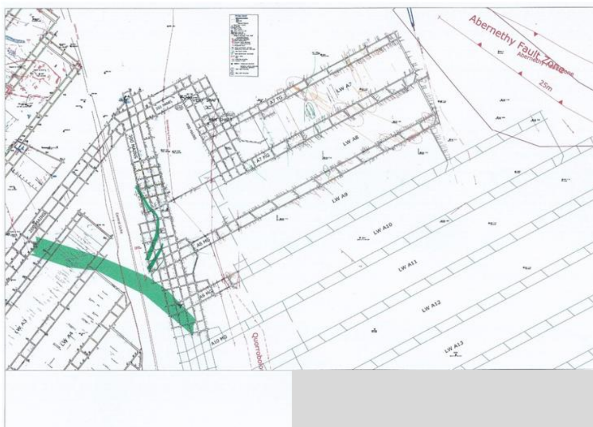
Figure 12. Structural geology features in the vicinity of Maingate A9
