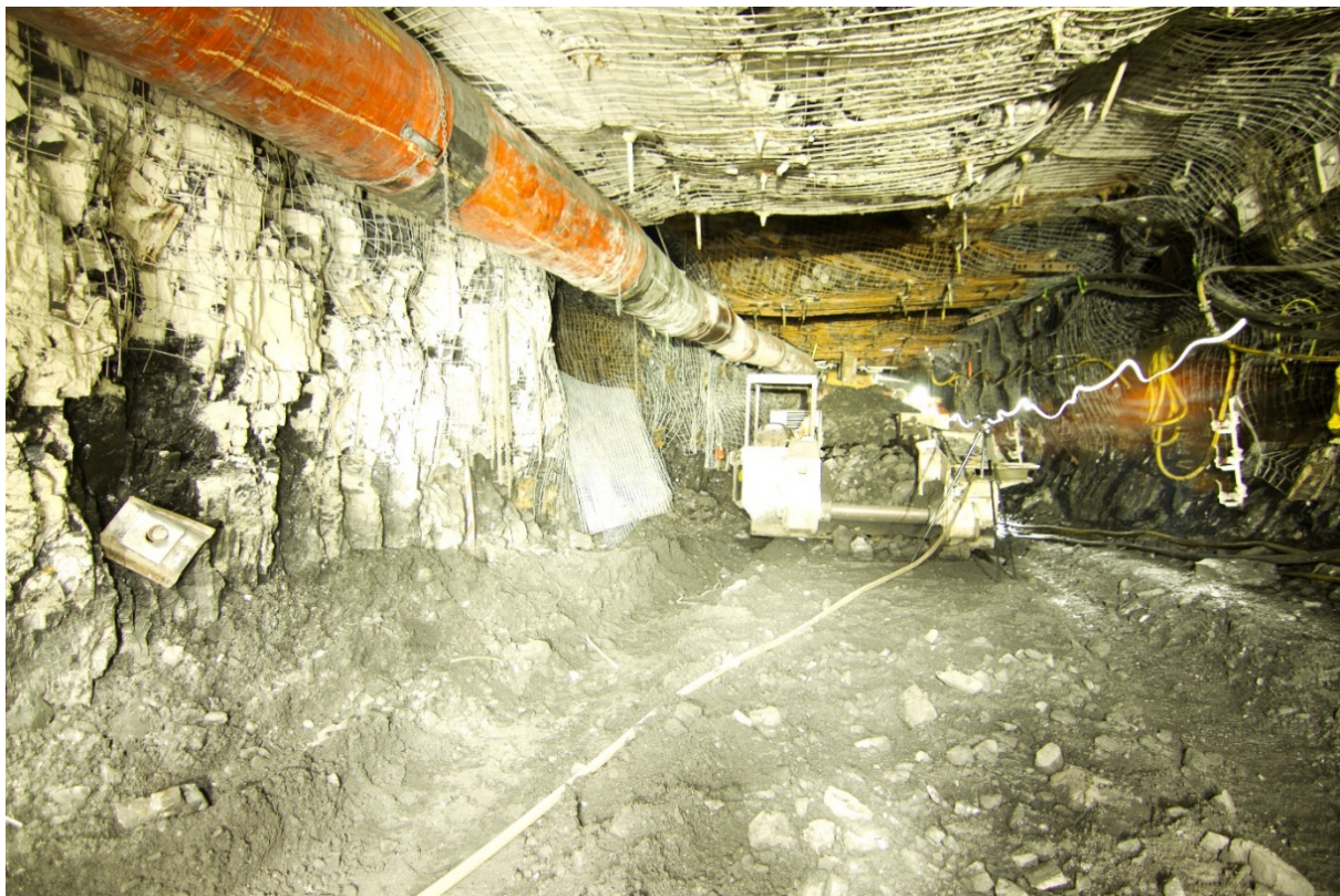
Figure 8: Close-up of burst coal pile adjacent to the continuous miner.
