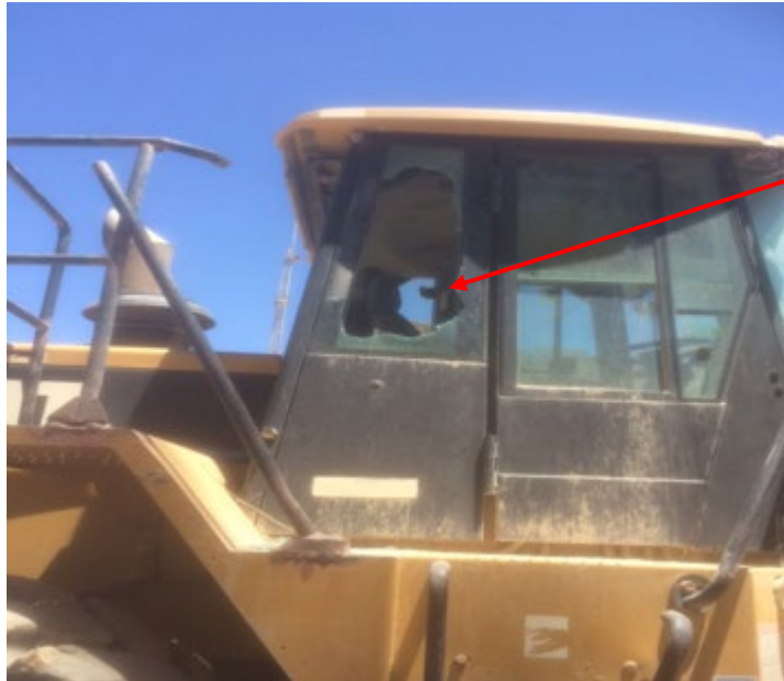
Figure 3 Equipment damaged by flyrock
