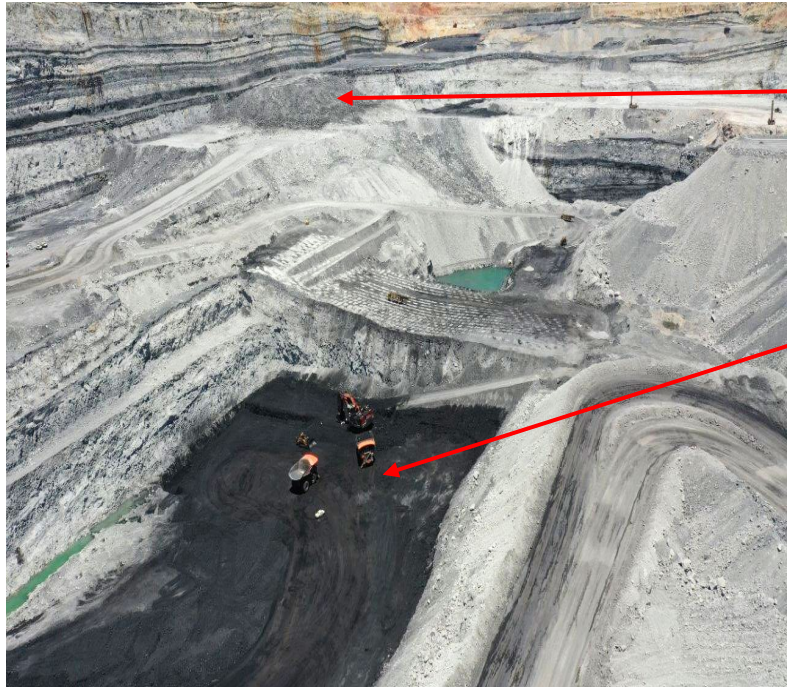
Figure 2 Flyrock contacts operating equipment from a blast
