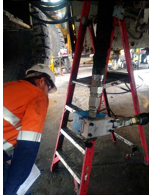
Figure 5: Disconnected hydraulic lines exiting from the excavator pod. The accumulator is hidden from view inside the base pod
