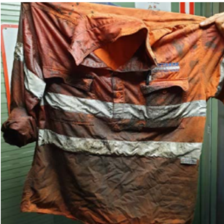
Figure 1: Shirt damaged by high pressure fluid release
