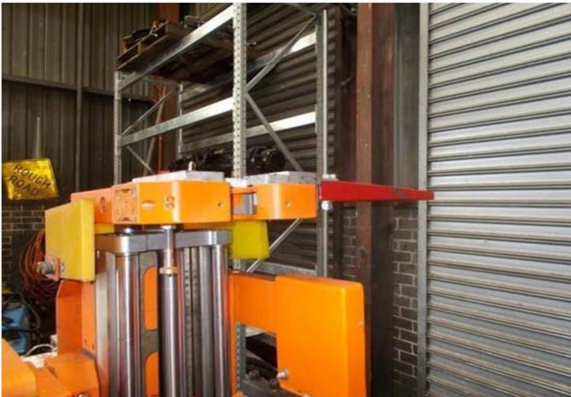
Cocky Beaks fitted to Bolting Rig
