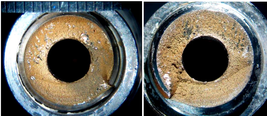
Figure 9- View of sample 2-1(Left) and sample 2-1-T (Right) fracture faces, consistent with brittle fracture over approximately 95% of the cross section followed by a shear lip.
