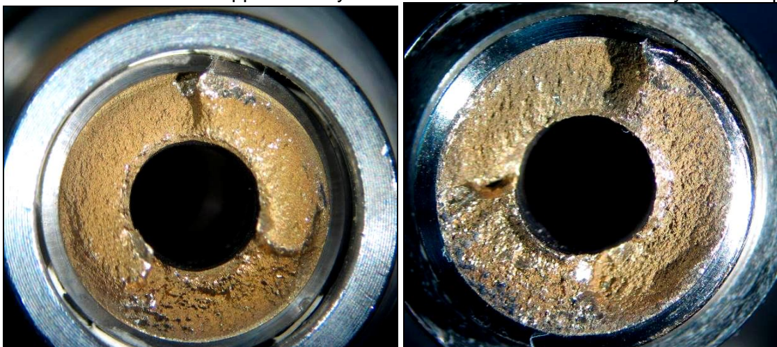
Figure 9- View of sample 2-1(Left) and sample 2-1-T (Right) fracture faces, consistent with brittle fracture over approximately 95% of the cross section followed by a shear lip.
