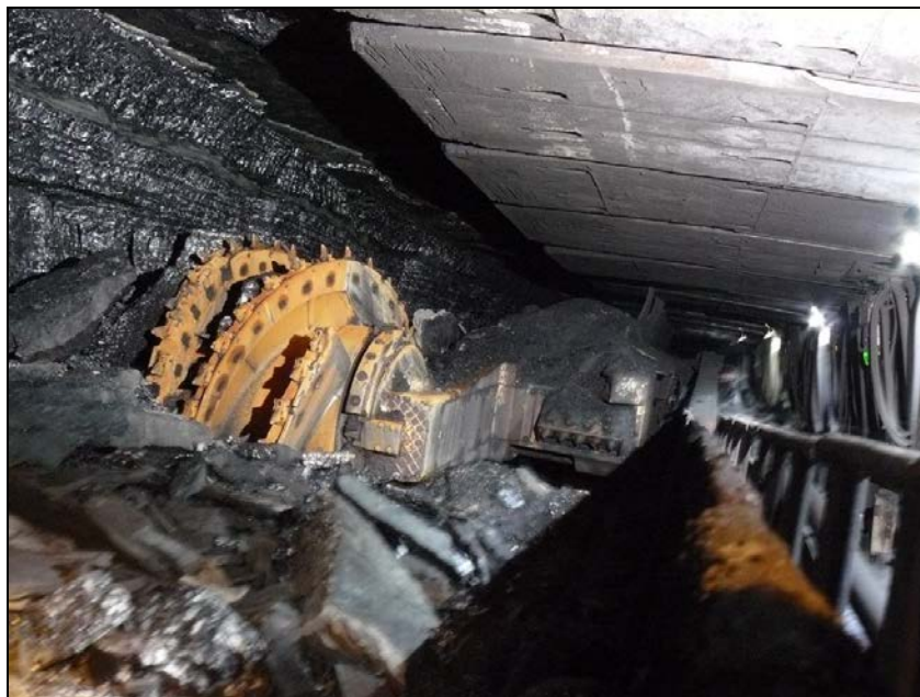
Figure 2: Longwall face Beltana Highwall mine showing shearer and longwall chocks
