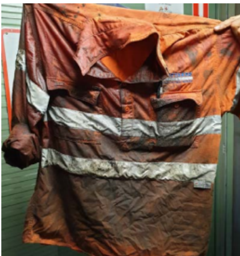
Figure 1: Shirt damaged by high pressure fluid release
