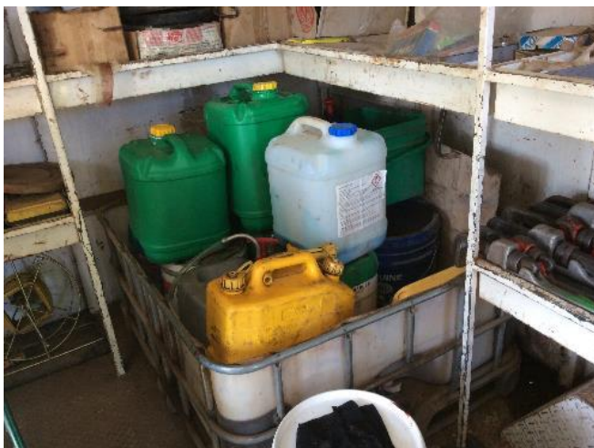
Figure 1 Chemicals and fuels stored on bunded pallet in drillers caravan
