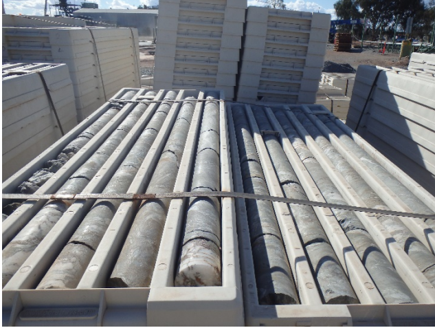
Figure 15 Core stored in modular plastic core trays
