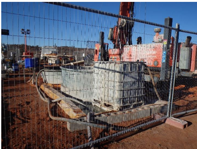
Figure 17 Use of banded aboveground sumps
