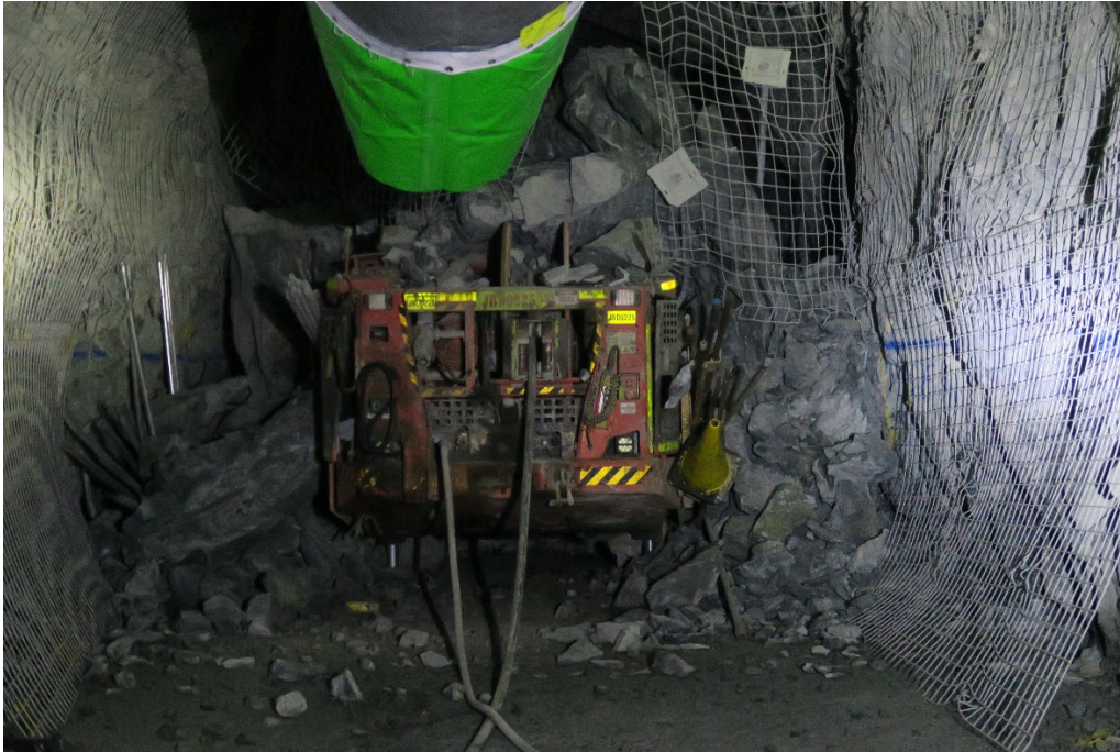
Figure 1: The jumbo drill rig partially buried by the roof collapse
