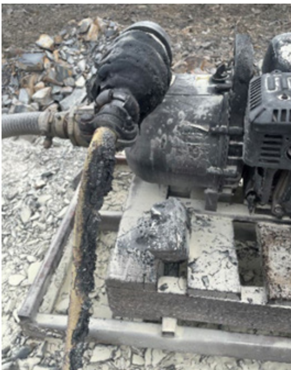
Picture 19. Charred pump after ignition incident
