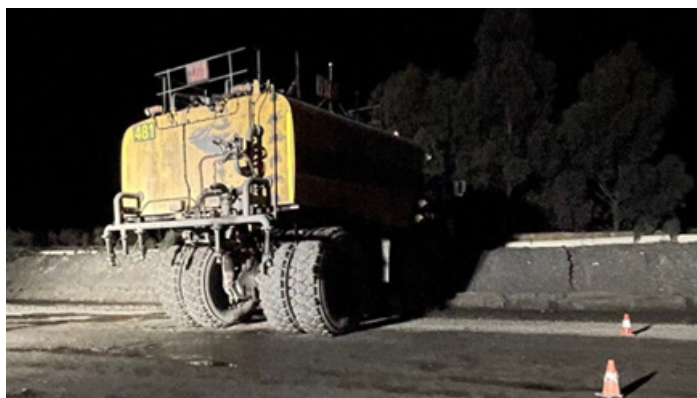
Picture 7. Water cart stopped on windrow
