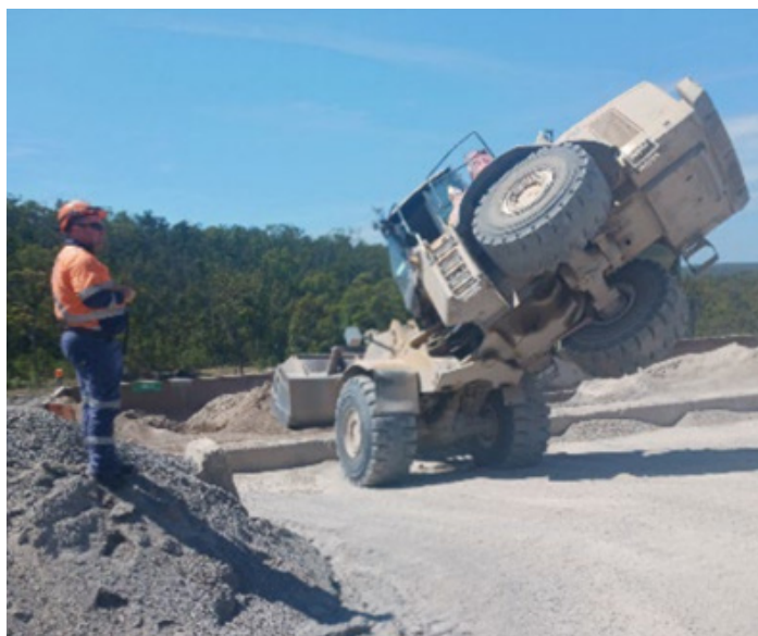
Picture 14. Stricken LHD with rear wheels off the ground
