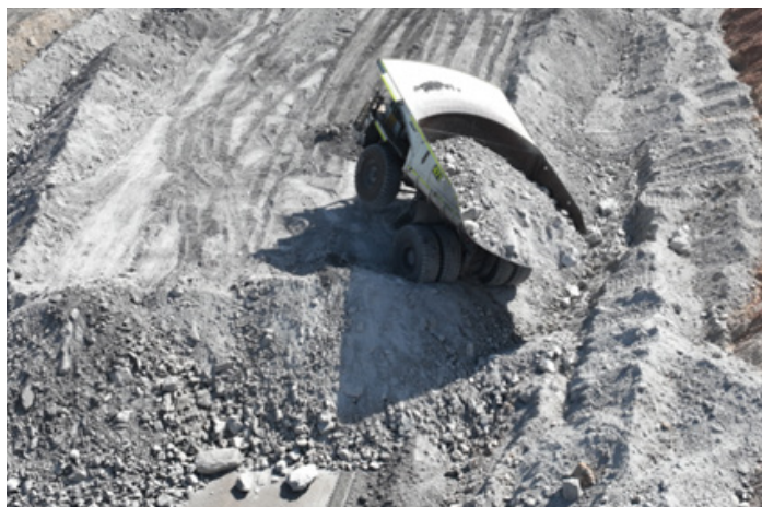
Picture 18. Slumped truck with raised wheel
