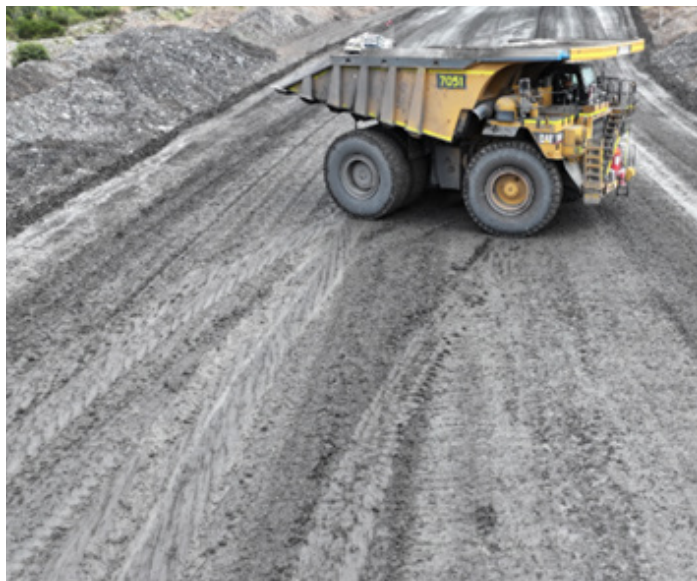
Picture 12. Dump truck spun on wet road
