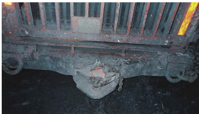
Picture 10. LHD collision damage
