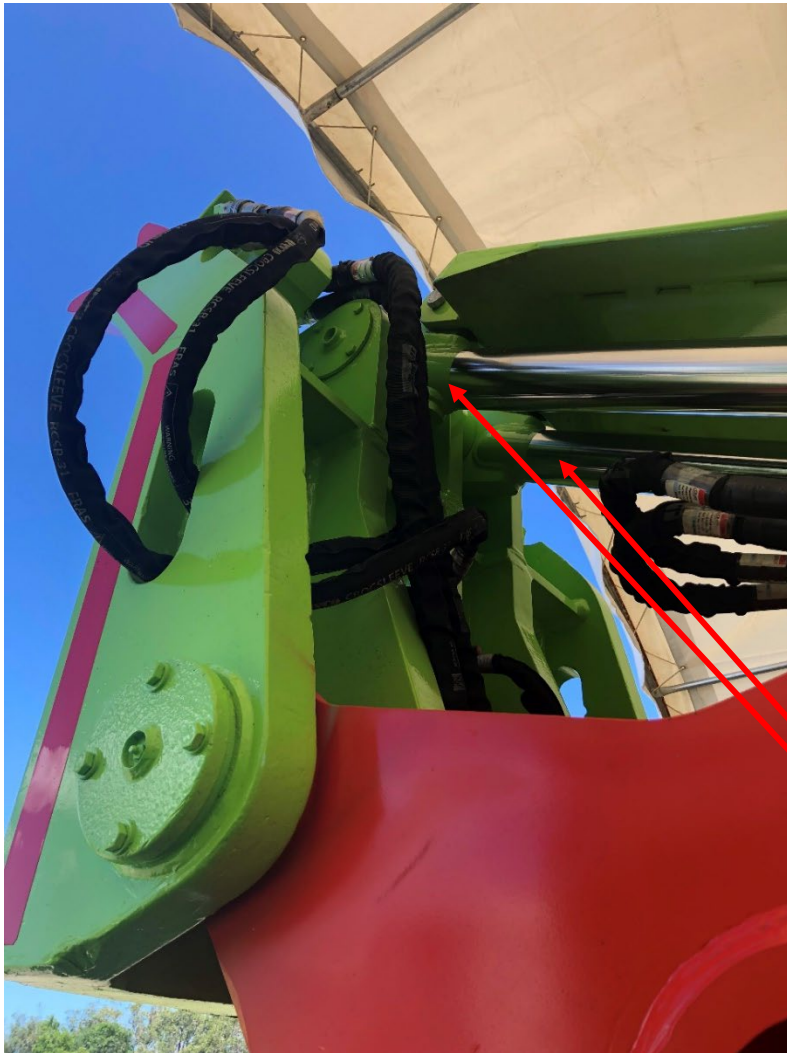
Figure 4: Photograph of a OEM development of a twin crowd cylinder on a underground coal LHD loader
