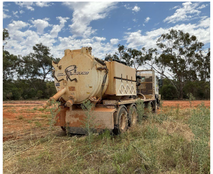
Figure 7: Liquid waste vacuum truck at TAKD142
