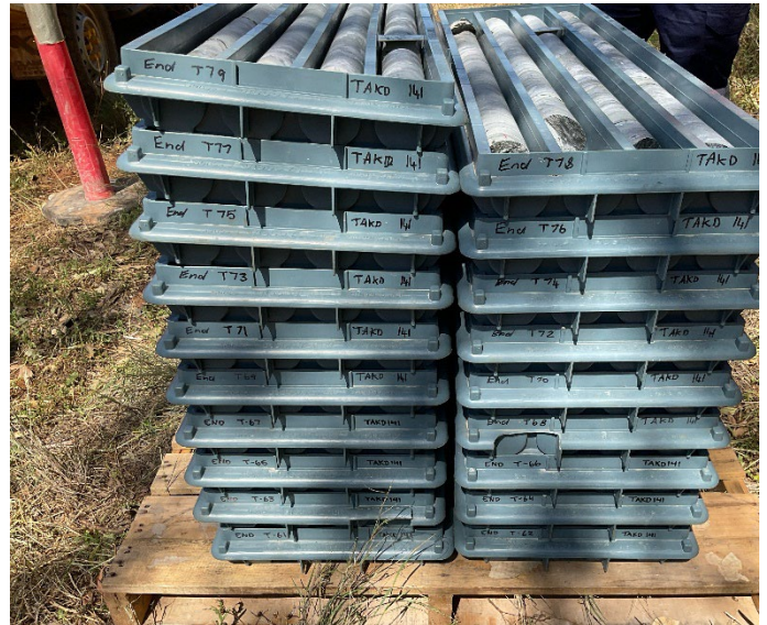
Figure 10: Core trays stacked and labelled at TAKD141
