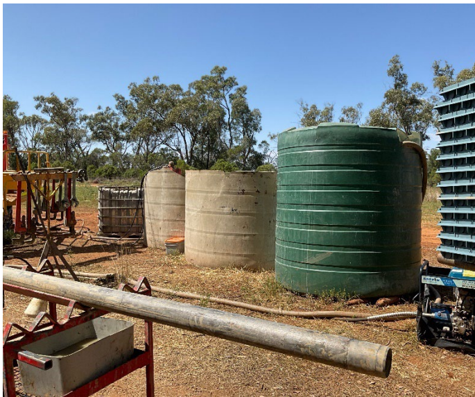
Figure 6: Above ground sumps at TAKD141
