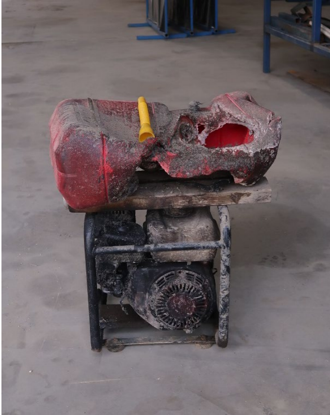
Figure 3: The fire-damaged water pump retrofitted with a 20 litre marine-grade plastic fuel container
