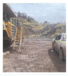
Parking near a haul truck without establishing positive communications can have fatal consequences and should not occur under any circumstances.
